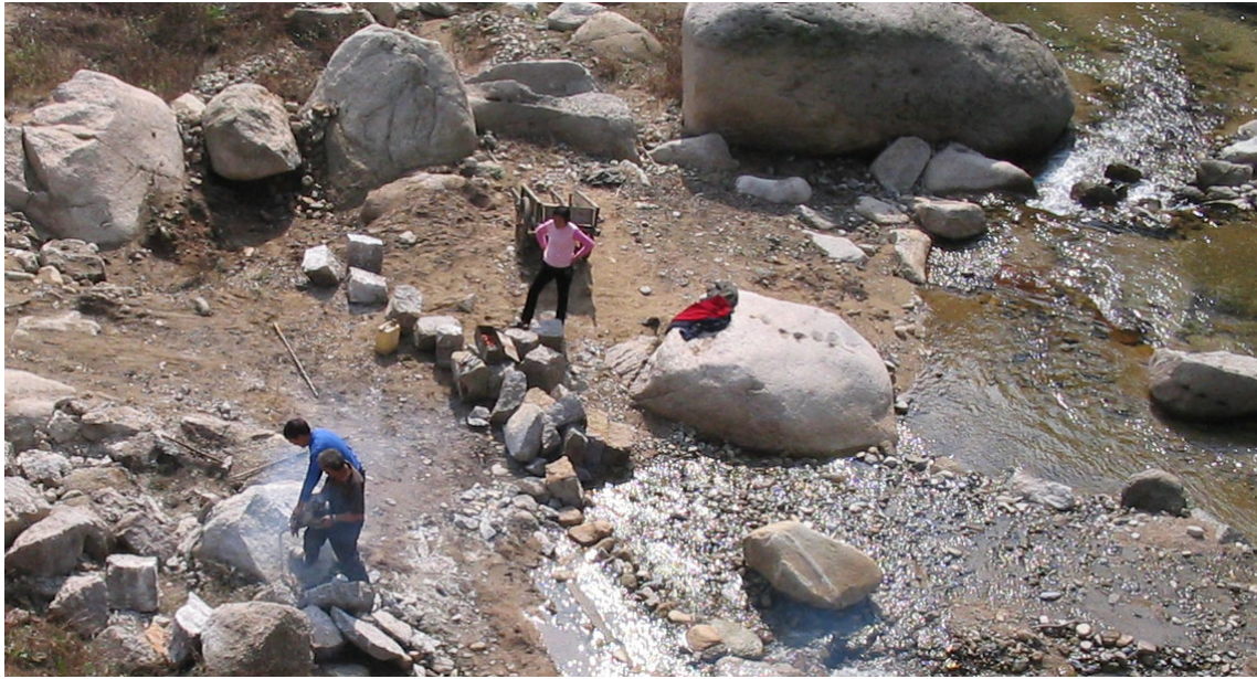
Plate 6. Villagers cut boulders in a local stream to make construction materials.
